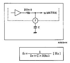
The value of the external capacitor connected to pin 7 determines the output signal frequency characteristics during HCC control.
