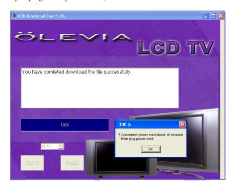
12. Press the OK button and exit the Interface Tool. Disconnect the USB cable from your TV/Computer.
