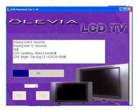
8. When step 1 is complete, a message will prompt you to disconnect and connect the power cord. (Press OK after you plug in the power cord.)
