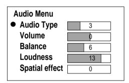
Use the  $P \bigvee$  or  $P \triangle$  buttons to select the option, then press the F/OK button on the remote control to enter.
