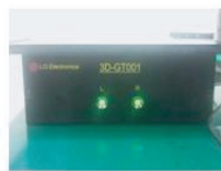
<IR Tester Lamp turned on(OK)>
