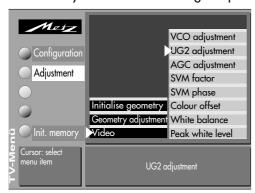
Press the **OK** key to display the Ug2 test pattern. Turn the screen-grid adjustment control Ug2 (the bottom control on the line transformer) fully counterclockwise and then turn it slowly clockwise until the red bar on the screen changes to green. Turn the control further until the bar changes back to red. Then turn the control back slightly until the bar changes back to green.
