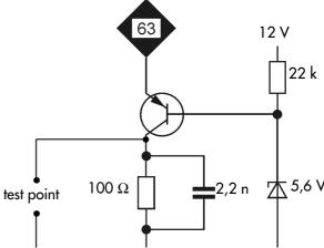
Connect an oscilloscope to the  $100 \Omega$  resistor of the measuring circuit
